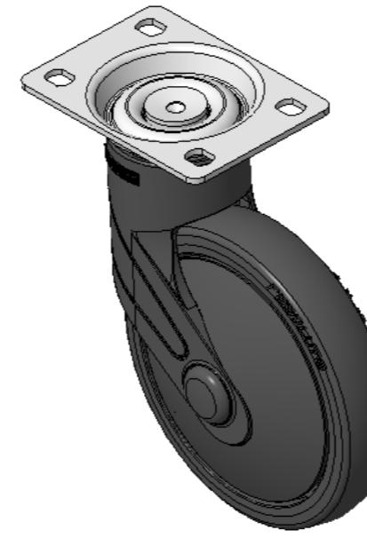
Wheel tread: Thermoplastic rubber elastomer (TPR)
